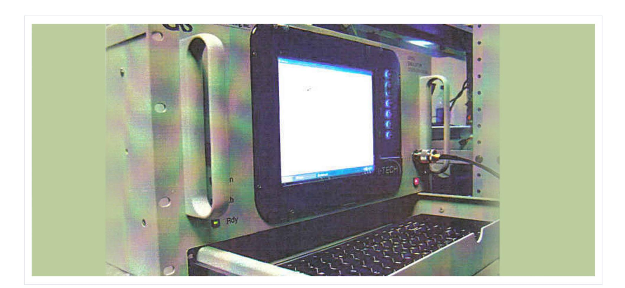
The Real Time Signal Intercept, Analysis and Countermeasure system provides an integrated system to capture wide band RF signals, perform real time analysis of the signal, and if necessary, take effective countermeasure. It performs most cognitive radio functions necessary for communication, navigation and radar surveillance, intercept, analysis, and countermeasure.
