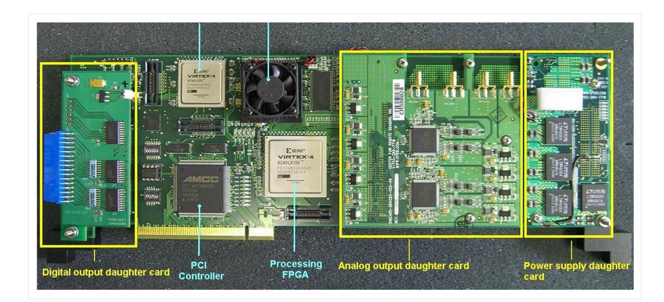
The PCI-DSP-FPGA series of boards provide advanced capabilities of using both DSPs and FPGAs enabling a variety of sequential and parallel processing tasks to be integrated in truly real-time operation. These boards provide enhanced functionalities over the PCI-DSP series.
