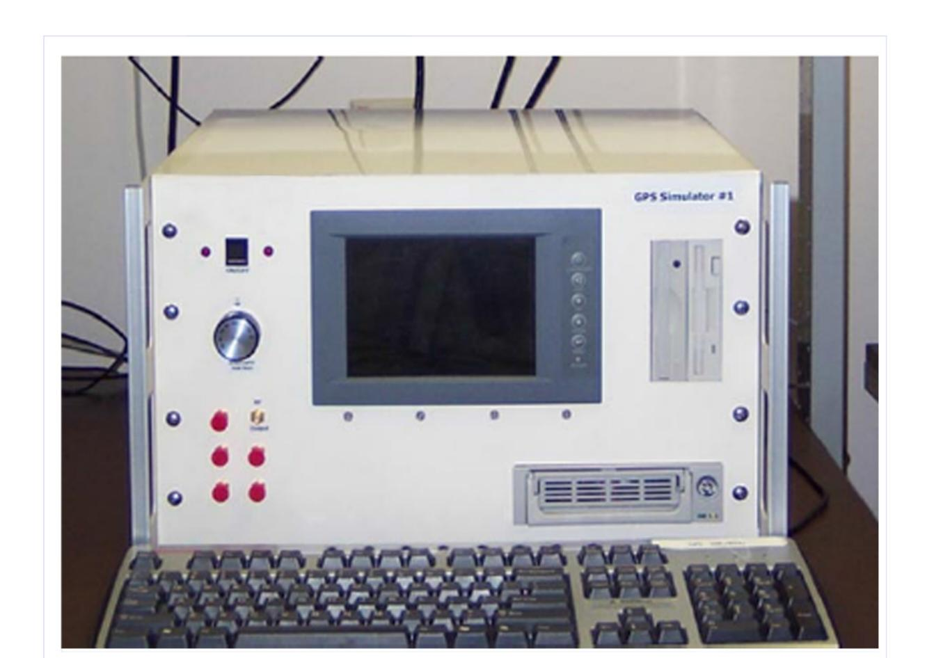
The GPS Signal Generator from CRS, Inc. provides live RF signals at navigational frequencies ( $L_1$ ,  $L_2$ , and  $L_5$ ) suitable for Hardware in the Loop (HWIL) signal generation.
