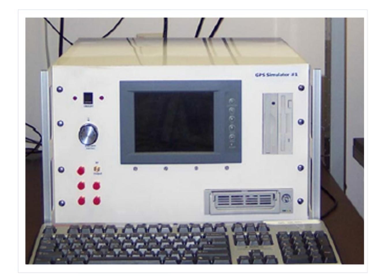
The GPS Signal Generator from CRS, Inc. provides live RF signals at navigational frequencies ( $L_1$  and  $L_2$ ) at two independent platforms suitable for precise, rover, and base station simulation.
