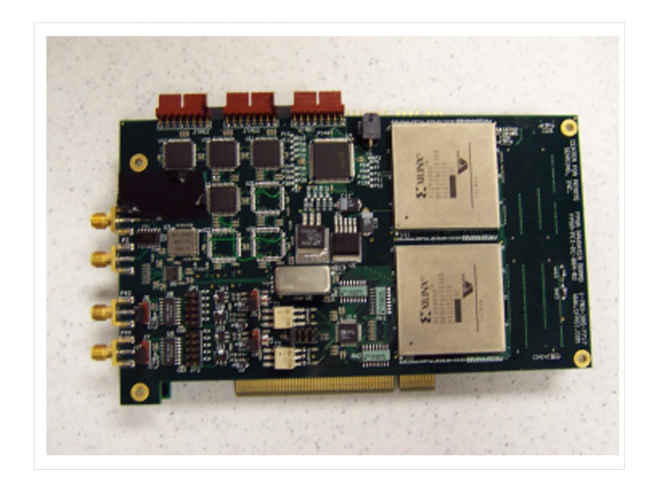
The PCI-FPGA series of boards provide versatility, ease of operation, and, most importantly, extremely high processing capacity achieved through dual Virtex II FPGAs in conjunction with the independent PCI interface.
